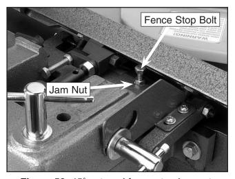
Figure 52. 45° outward fence stop jam nut.
